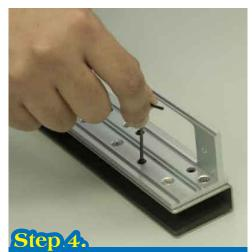
Screw Allen screw into plug box (This Allen screw is used to tighten glass, so you may just screw in a little bit)
