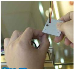
Step 13. Pull out the bolt lock wire from wire hole
