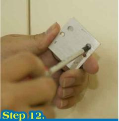
Use screwdriver to punch wire hole on side cover.
