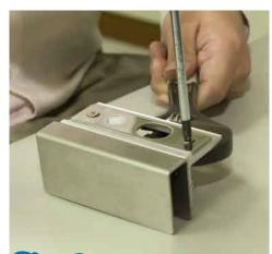
Step 9. Screw the strike plate on short plug box
