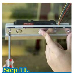
Install the bolt lock into plug box.
