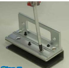
Step 7. Screw short plug box on short U-bracket.
